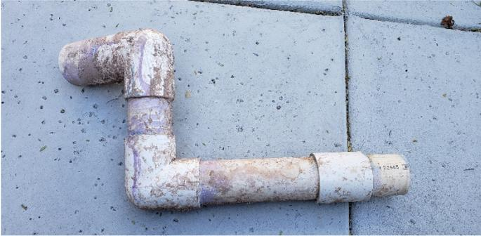
*Failed supply pipe due to improper use of glued joints*
